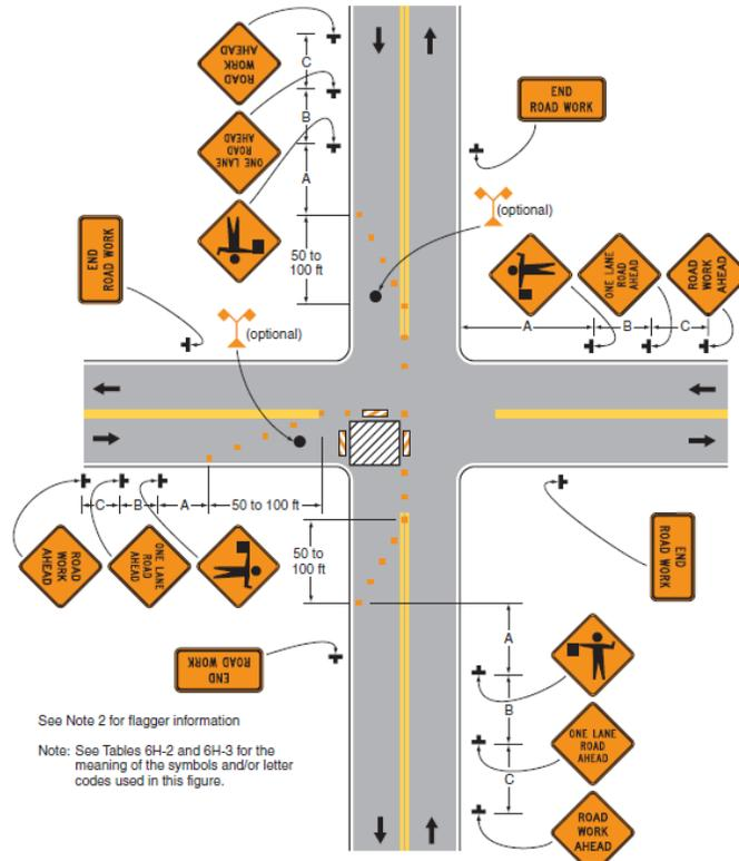
**Figure 2.7 Closure at the Side of an Intersection**
