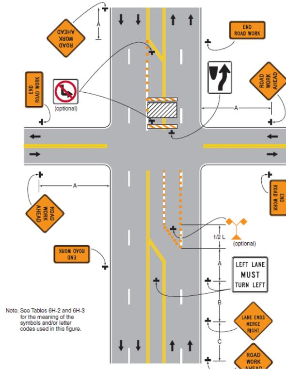
**Figure 2.5 Multiple Lane Closures at an Intersection**
