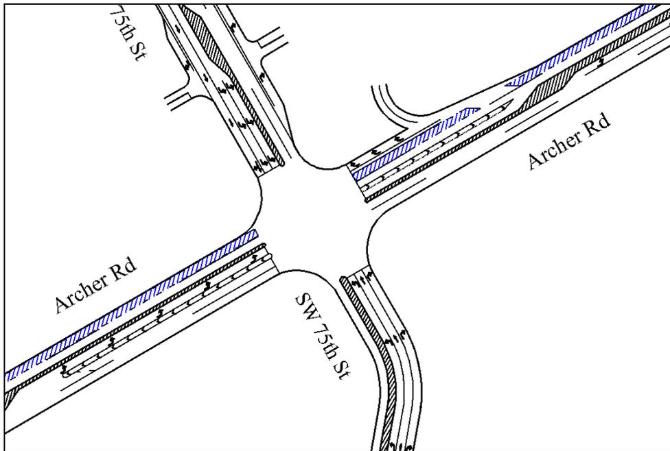
**Figure 5.3 Sketch of the Lane Closure in Westbound for the Intersection of Archer Rd and SW 75<sup>th</sup> St.**
