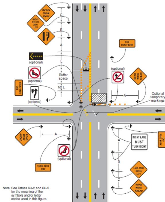
**Figure 2.4 Half Road Closure on the Far Side of an Intersection**
