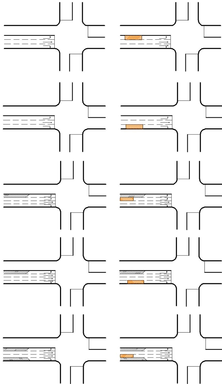
**Figure 2.9 Lane Closure Affects a Turning Movement**
