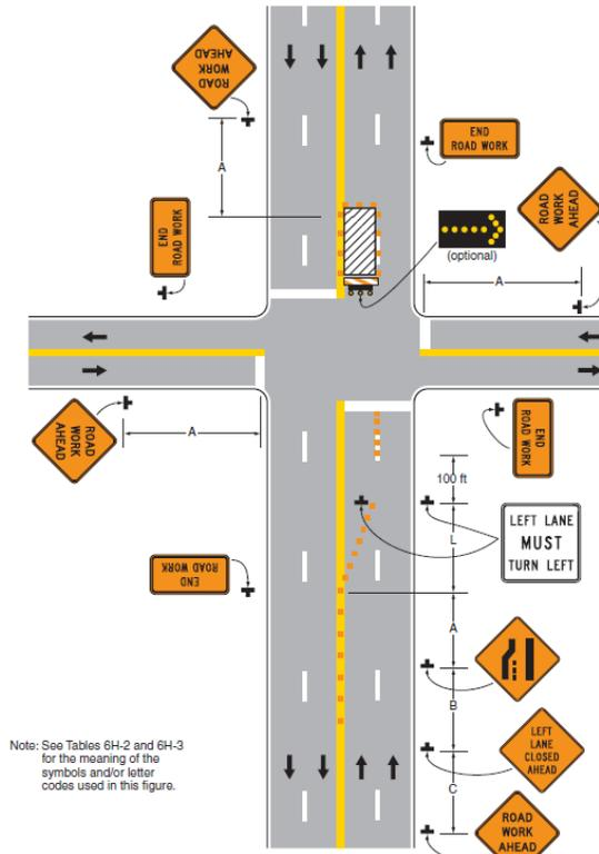
**Figure 2.3 Left-Hand Lane Closure on the Far Side of an Intersection**
