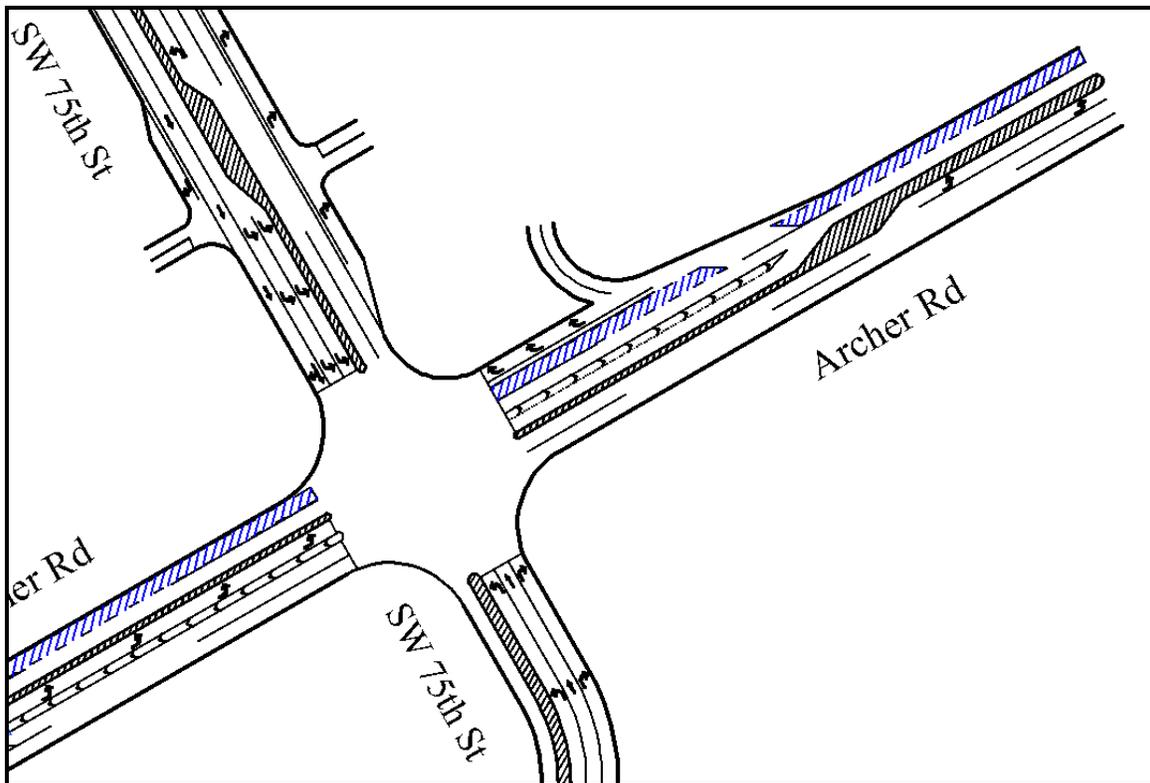
**Figure 4.3 Sketch of the Lane Closure in Westbound Archer Rd at the Intersection of Archer Rd and SW 75<sup>th</sup> St**
