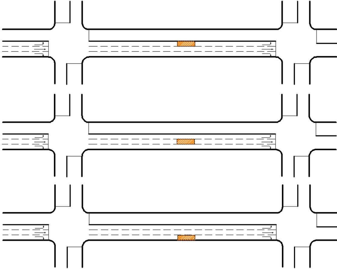
**Figure 2.16 Lane Closure at Some Distance Downstream from the Subject Intersection**
