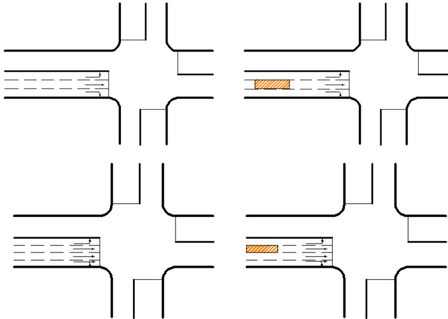
**Figure 2.10 Lane Closure Affects the Through Movement**
