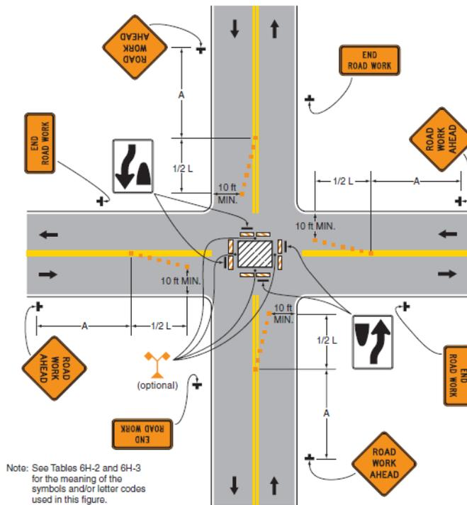
**Figure 2.6 Closure in the Center of an Intersection**
