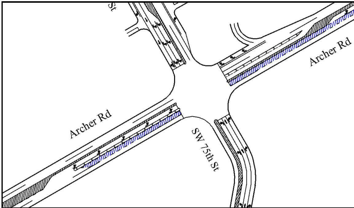
**Figure 4.4 Sketch of the Lane Closure in Eastbound Archer Rd at the Intersection of Archer Rd and SW 75<sup>th</sup> St**
