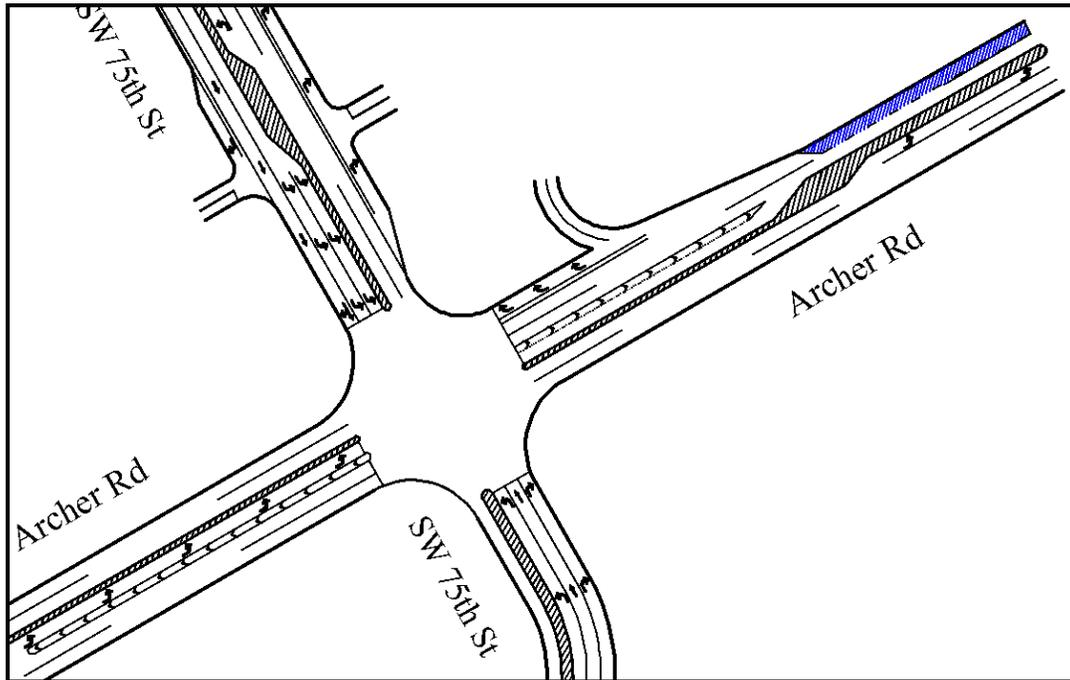
**Figure 5.1 Sketch of the Lane Closure in Westbound Archer Rd before the Intersection of Archer Rd and SW 75<sup>th</sup> St.**
