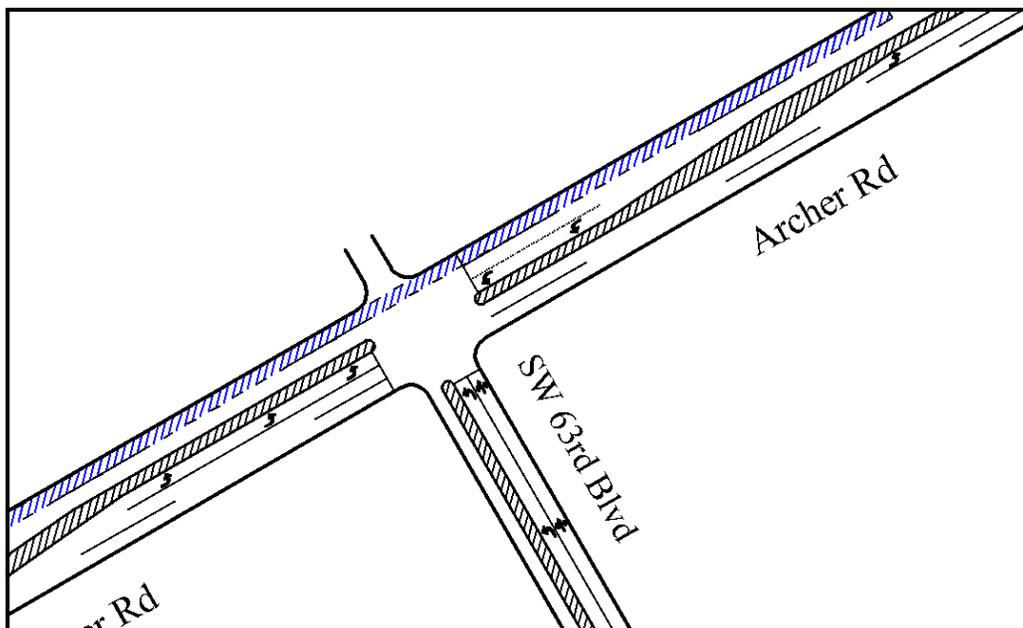
**Figure 5.4 Sketch of the Lane Closure in Westbound for the Intersection of Archer Rd and SW 63<sup>rd</sup> Blvd**
