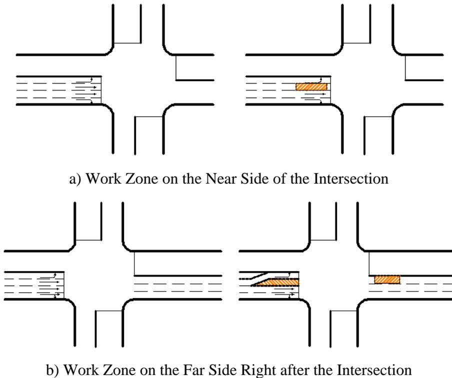
**Figure 3.8 Case 2: Lane Closure at the Stop Bar**
