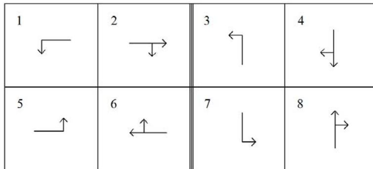
**Figure 3.6 Phasing Diagram of the Study Intersection**
