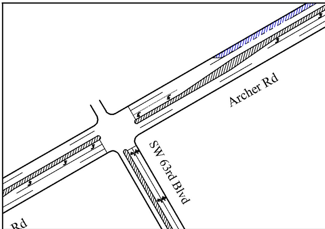
**Figure 5.2 Sketch of the Lane Closure in Westbound Archer Rd before the Intersection of Archer Rd and SW 63<sup>rd</sup> Blvd**
